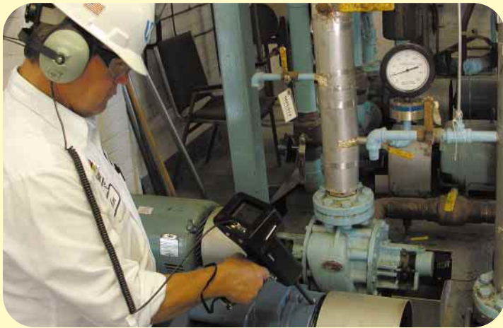
Ultrasound inspection provides bearing information through headphones, as intensity readings on a meter/display panel or on a recording device such as a portable PC or portable vibration analyzer.
