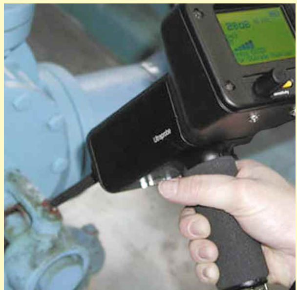
Ultrasound inspection of bearings provides early warning of potential failure and helps determine if a bearing needs lubrication.
