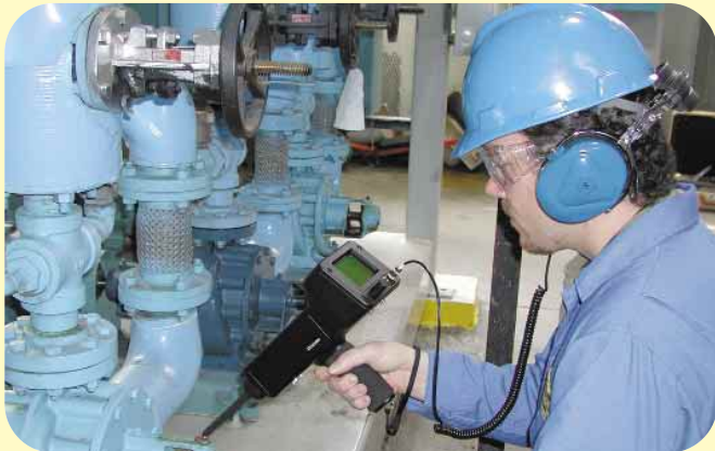
The high frequency, short wave characteristic of ultrasound allows the signal to be isolated so that a user can hear and determine if a bearing is malfunctioning.
